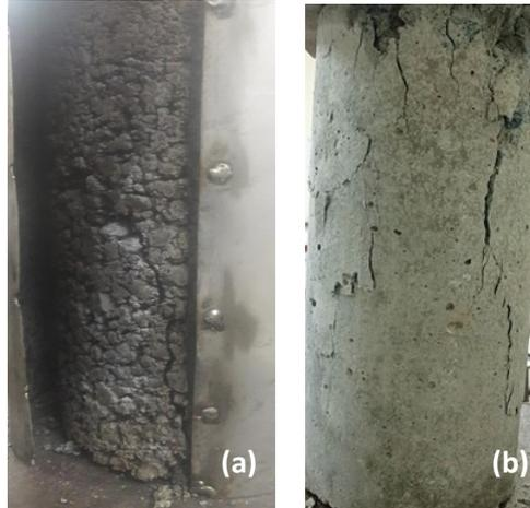
Figure 2. Cracks in column members(a) Diagonal Cracks (b) Splitting Cracks
