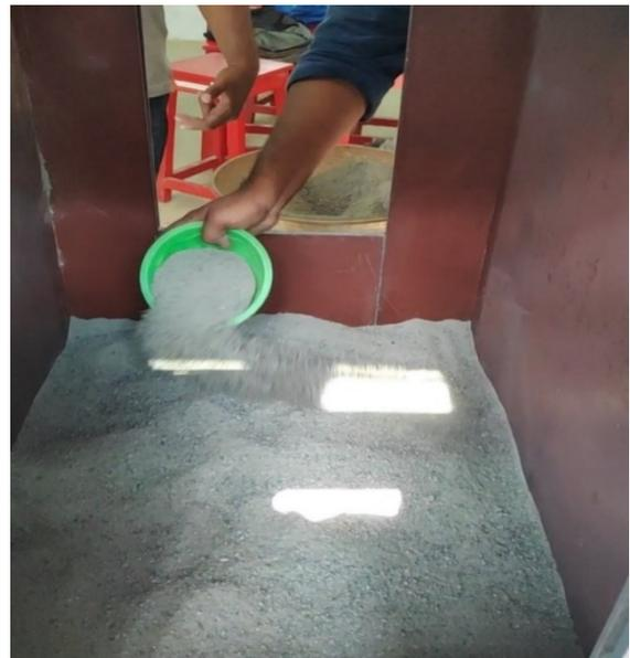
Figure 9. Filling of loose M-Sand bed
