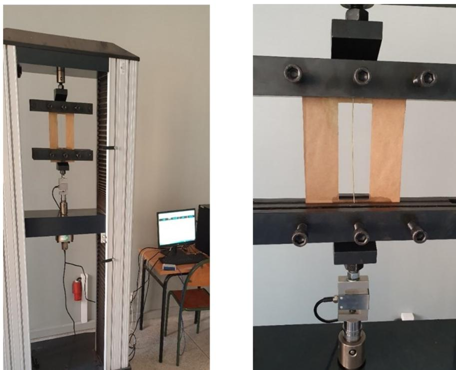
Figure 4. Tensile testing of Alfa fiber
