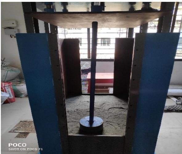
Figure 8. Compacted a dense M-Sand bed
