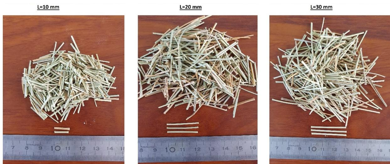
Figure 1. Cut Alfa fiber
