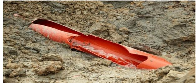
Figure 1. Failure due to deflection
