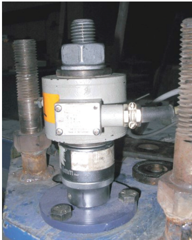
a) Setup for preload force measurements
