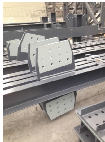
b) Flying surface in gusset plate
