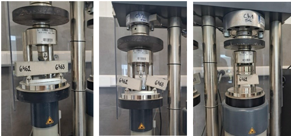
Figure 2. Testing of the mortar specimen
