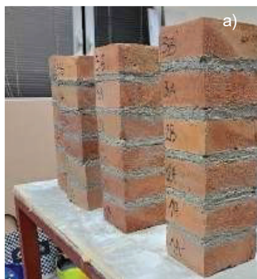
Figure 5. Preparation of the specimens (group III): a) masonry elements, b) area to be strengthened, c) FRCM system applied on masonry element with overhang fabric
