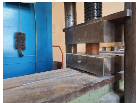
Figure 4. Preparation and testing of brick specimens
