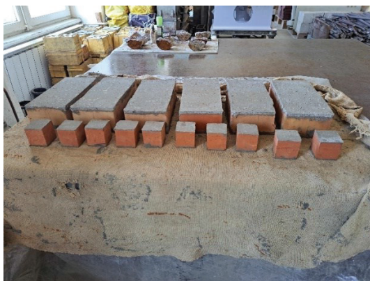
Figure 4. Preparation and testing of brick specimens
