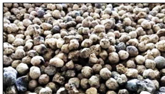
Figure 3. Typical View of Sintered Fly ash Aggregates
