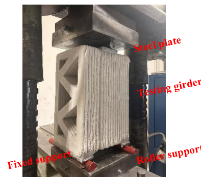
Figure 9. Experimental setup for 3-point test for individual segment
