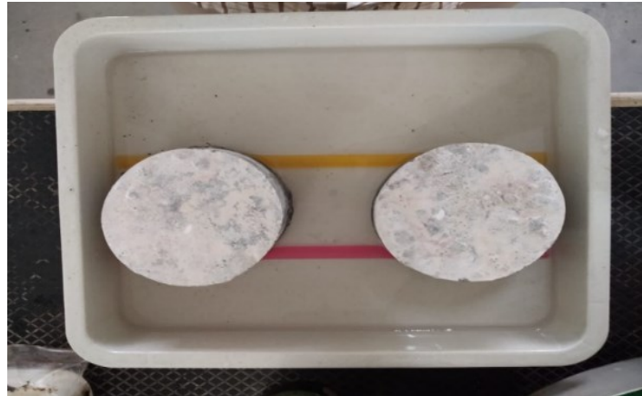
Figure 19. Test Setup for Sorptivity of Concrete Cylindrical Specimens
