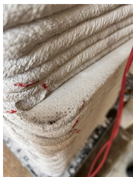
Figure 17. The local destruction of segments
