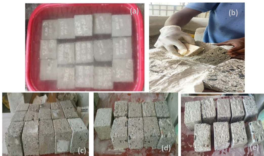
Figure 6(a). Cubes immersed in sulphuric acid (b) removing of loose materials with metal brush (c) Immersed cubes on 3 rd day (d) Immersed cubes on 7 th day (e) immersed cubes on 14 th day
