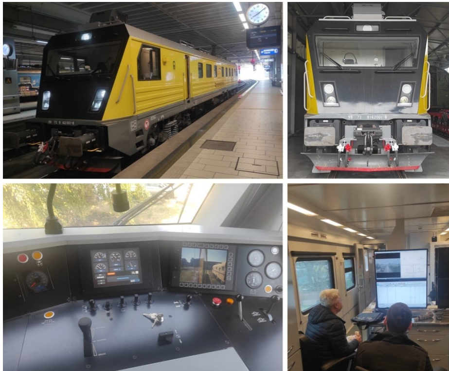
Figure 8. Modern recording car for track inspection on the Serbian railway network
