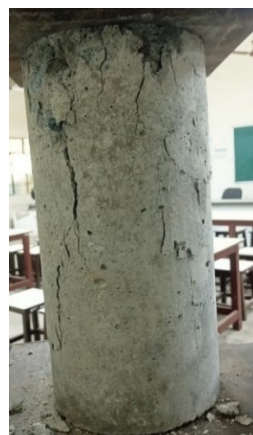
Figure 13. Tested specimen for Modulus of elasticity
