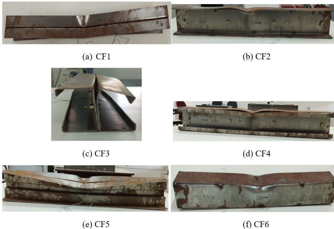
Figure 3. Tested CFS built-up beams
