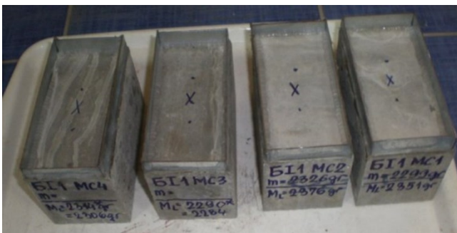
Figure 5. SCC-NRA surface appearance before testing
