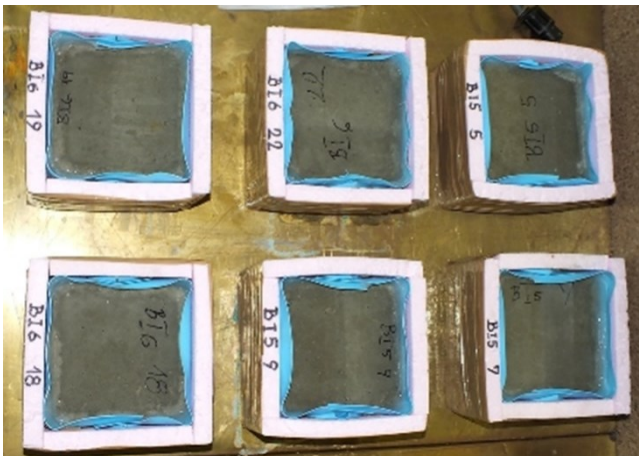
Figure 13. SCC-RCA-N and SCC-RCA-A surfaces appearance before testing
