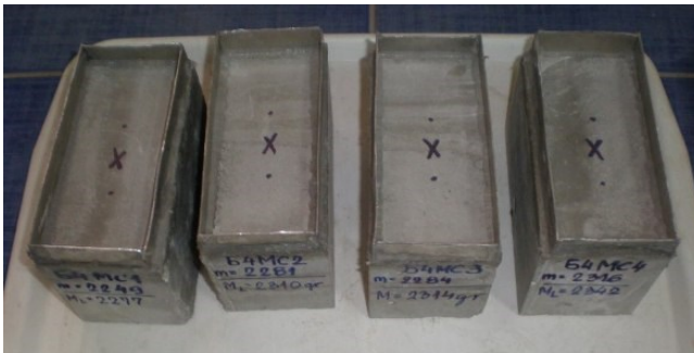
Figure 11. SCC-NMA-II surface appearance before testing
