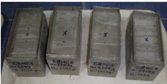
Figure 7. SCC-NCA surface appearance before testing
