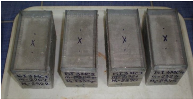
Figure 9. SCC-NMA-I surface appearance before testing
