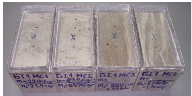
Figure 6. SCC-NRA surface appearance after 25 f/t cycles with de-icing salt
