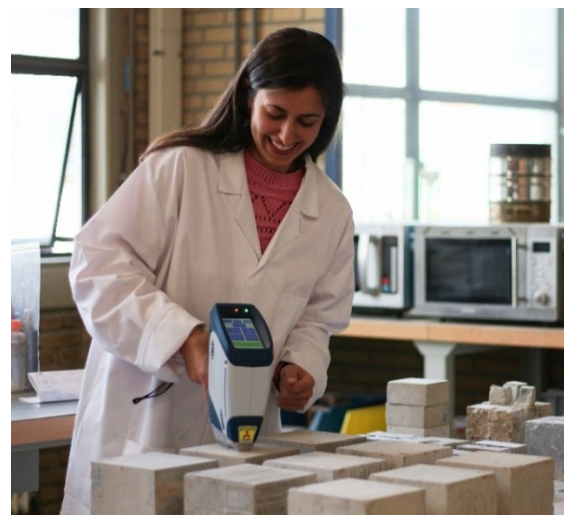
Fig. 12. The use of hXRF BRUKER device
