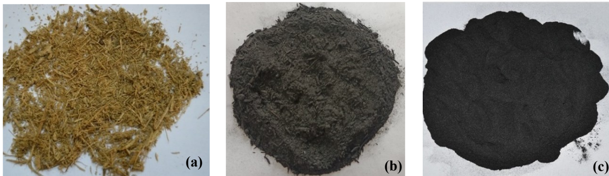
Figure 1. (a) Sugarcane fiber (b) burnt bagasse ash (c) sieved bagasse ash
