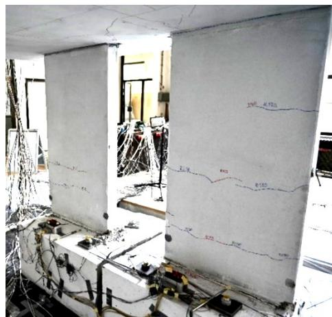
Figure 10. a) Cracks, which were observed in the wall piers,
