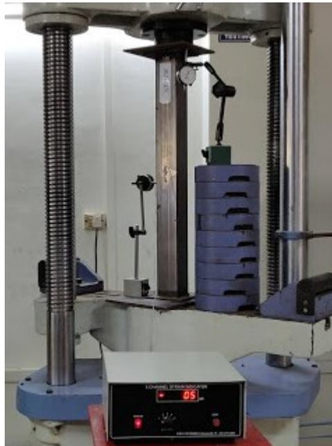
Fig. 3. Test set-up of the CFS wrapped column specimen
