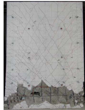
b) Crack pattern typical for cantilever walls
