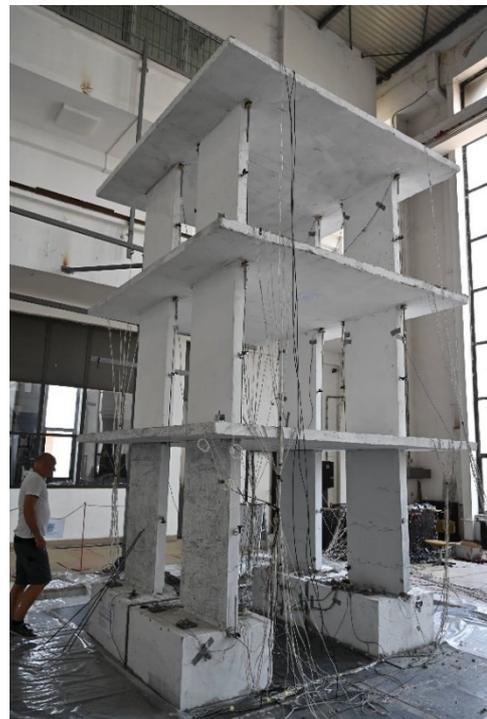
Figure 4. The tested specimen
