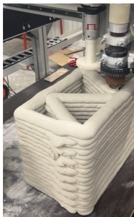
Figure 5. The process of 3DCP of individual segments
