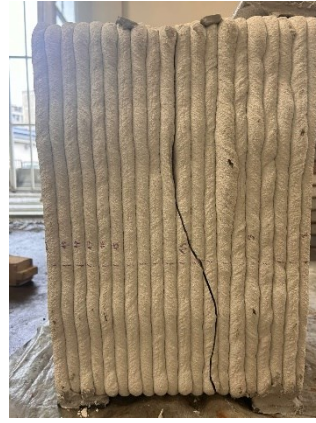
Figure 11. The failure mechanism of the segment in 3-point test - outside
