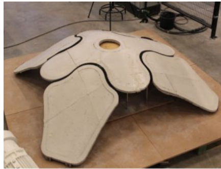
Figure 3. Horizontally printed panel [1]
