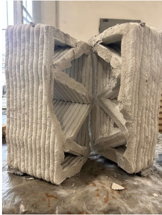
Figure 10. The failure mechanism of the segment in 3-point test - inside
