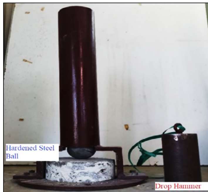
Figure 16. Test Setup for Drop Weight Impact Tester
