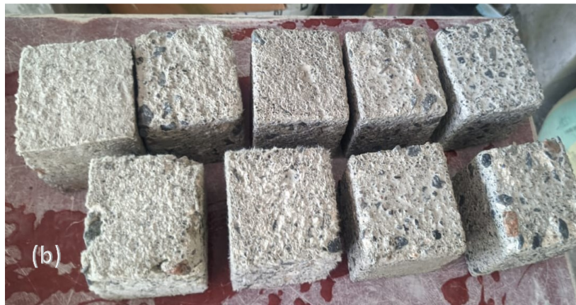
Figure 15. Acid attack specimen after (a) 7 days and (b) 14 days
