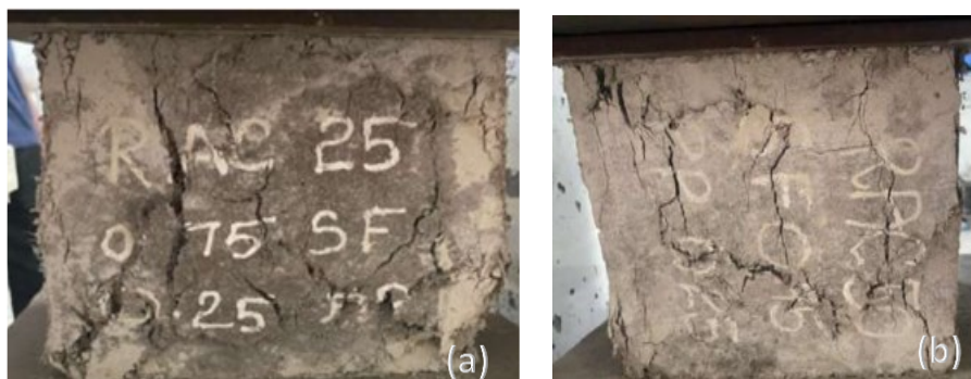
Figure 9. Formation of micro cracks in hybrid fiber reinforced recycled aggregate concrete (a) 25% RAC & (b) 50% RAC
