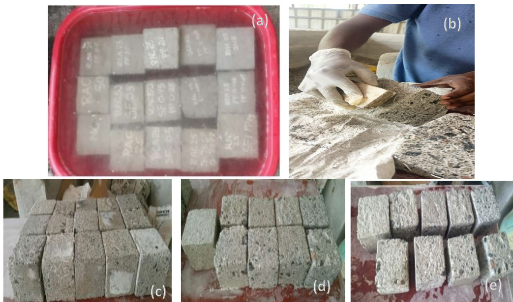
Figure 6(a). Cubes immersed in sulphuric acid (b) removing of loose materials with metal brush (c) Immersed cubes on 3 rd day (d) Immersed cubes on 7 th day (e) immersed cubes on 14 th day
