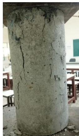
Figure 13. Tested specimen for Modulus of elasticity
