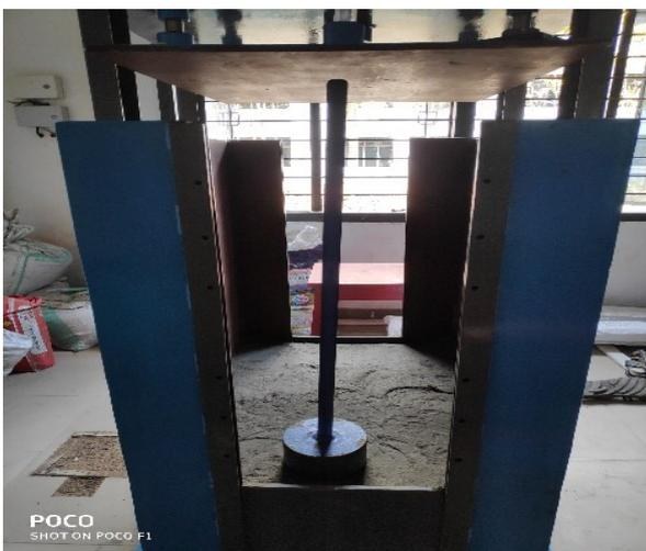
Figure 8. Compacted a dense M-Sand bed
