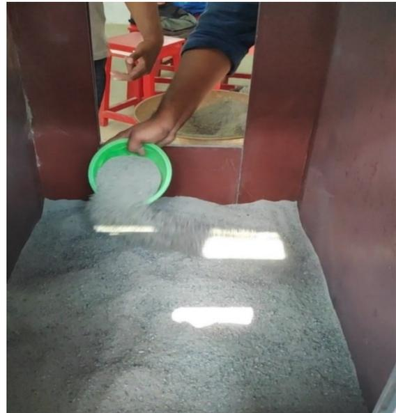
Figure 9. Filling of loose M-Sand bed
