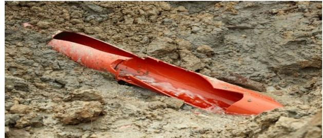
Figure 1. Failure due to deflection
