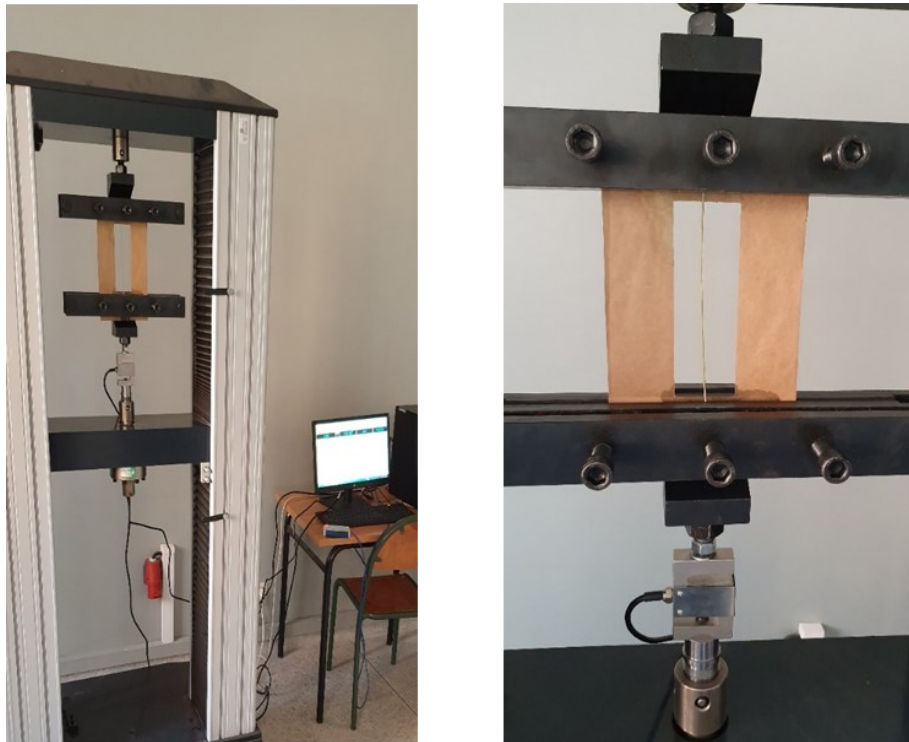
Figure 4. Tensile testing of Alfa fiber
