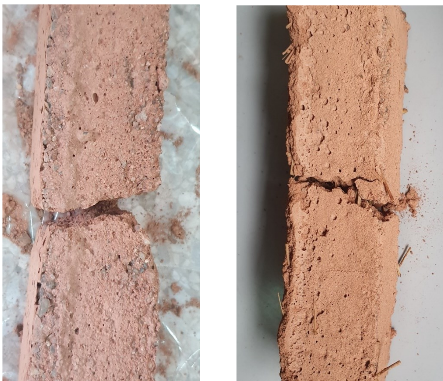
Figure 9. From left to right, unreinforced and reinforced sample after breaking
