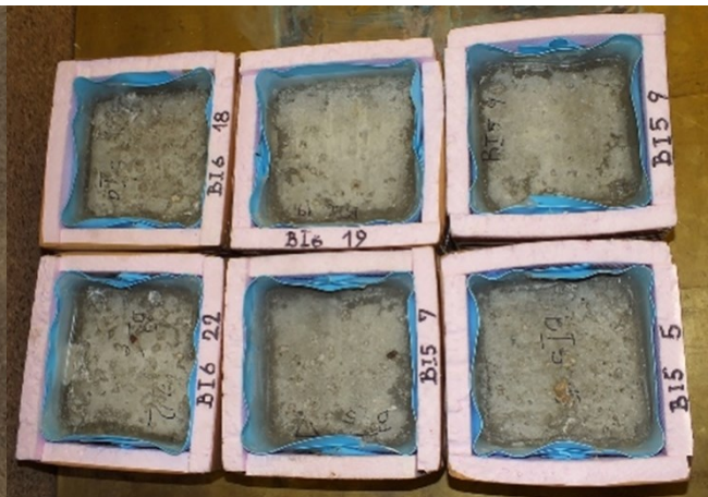
Figure 14. SCC-RCA-N and SCC-RCA-A surfaces appearance after 25 f/t cycles with de-icing salt
