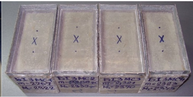
Figure 10. SCC-NMA-I surface appearance after 25 f/t cycles with de-icing salt
