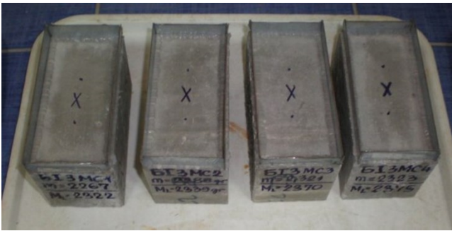
Figure 9. SCC-NMA-I surface appearance before testing
