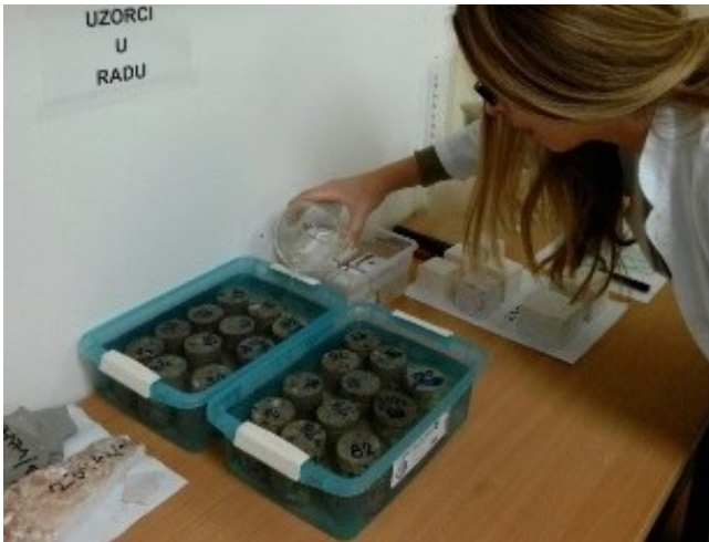
Figure 3. Water absorption by the test of gradual immersion at atmospheric pressure
