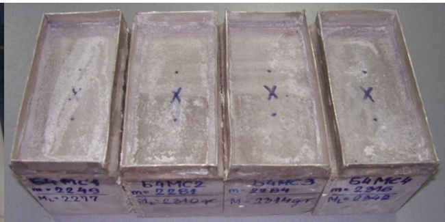
Figure 12. SCC-NMA-II surface appearance after 25 f/t cycles with de-icing salt
