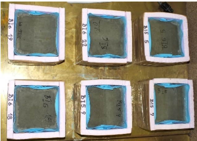
Figure 13. SCC-RCA-N and SCC-RCA-A surfaces appearance before testing
