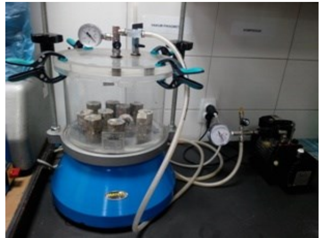
Figure 4. Water absorption by vacuuming
