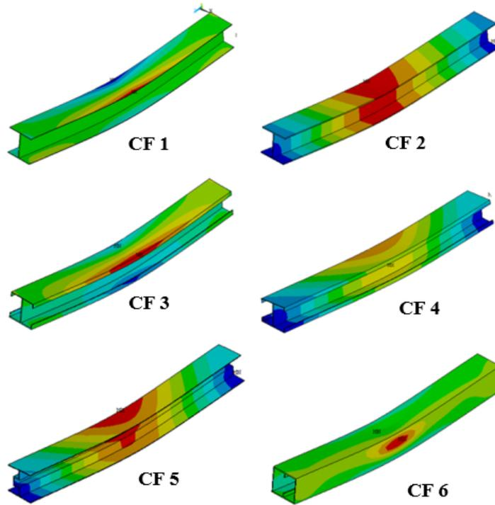
Figure 5. Deformed shape of the CFS built-up beams
