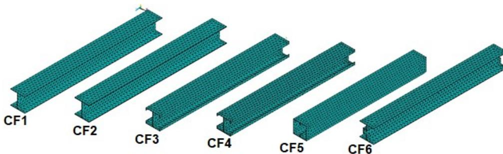
Figure 4. Mesh models of CFS built-up beams
