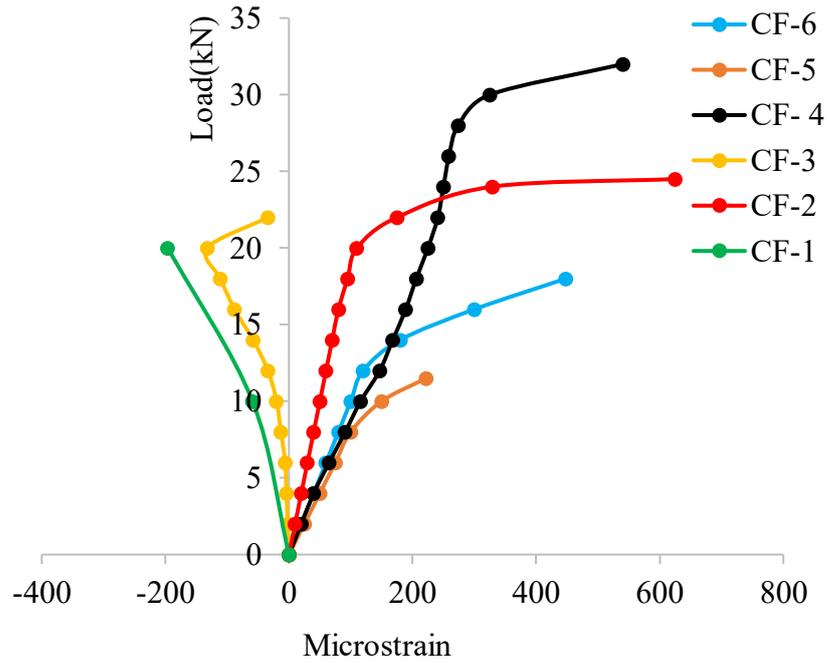
Figure 9. Load- strain behaviour of CFS built-up beams
