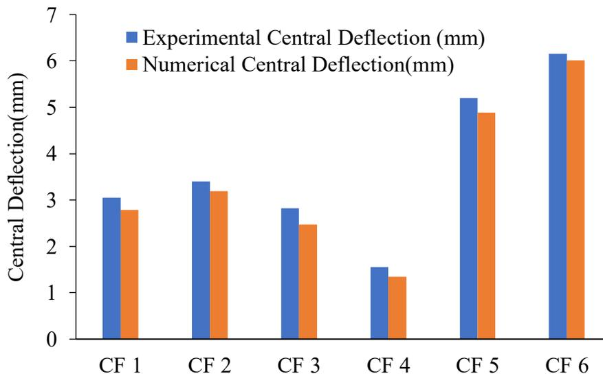
Figure 8. Bar chart comparison of the maximum central deflection
