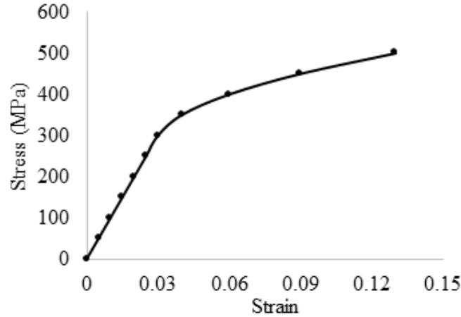
Figure 1. Stress - strain behaviour of the CFS material
