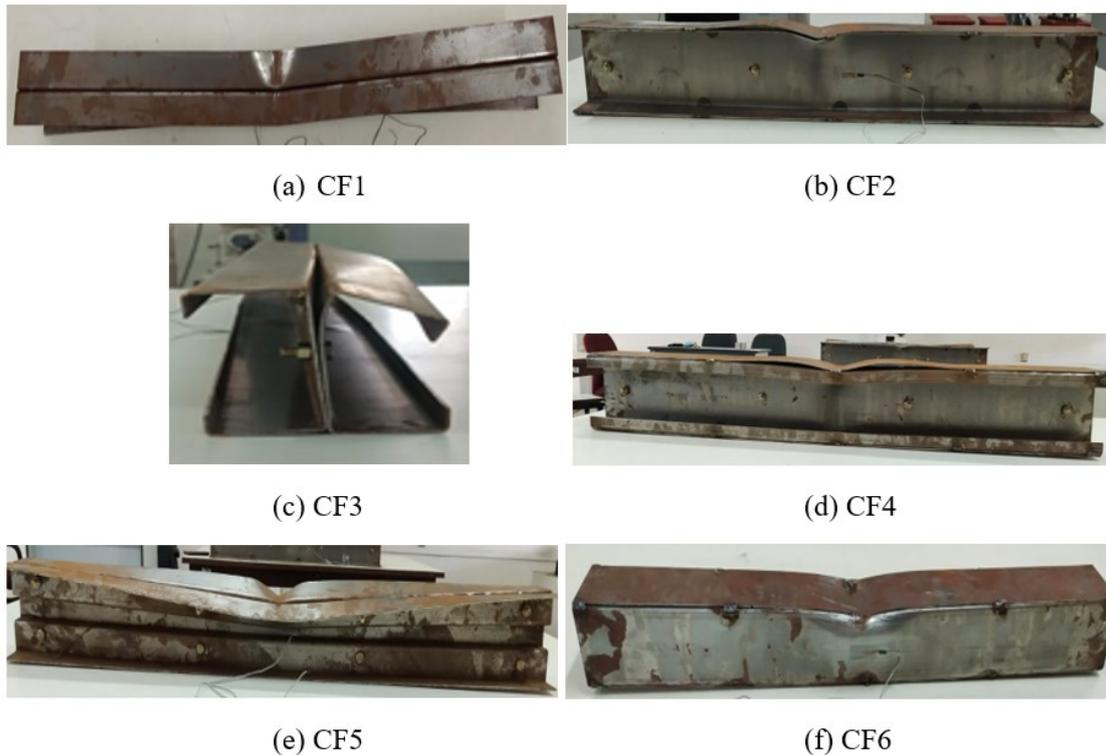
Figure 3. Tested CFS built-up beams
