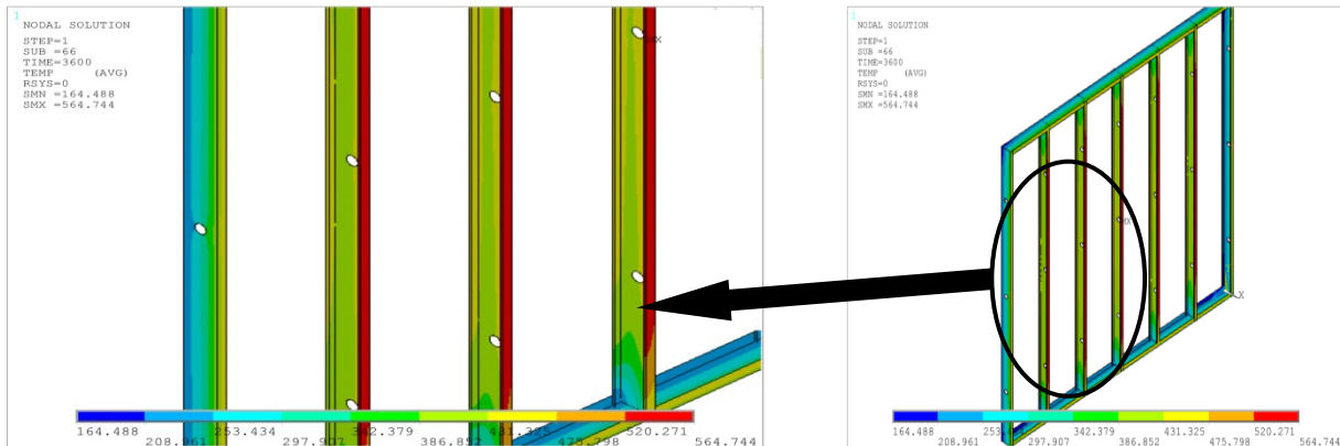
Figure 11. Temperature contours of model 2 at 60 minutes
