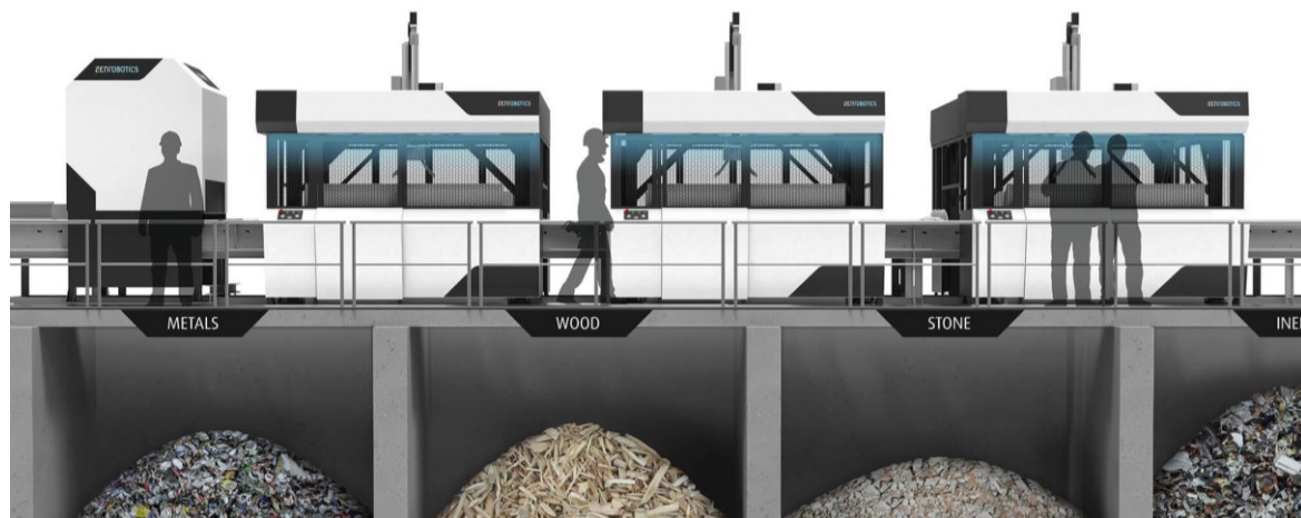
Fig. 3. ZenRobotics technology heavy picker sorting line [23]
