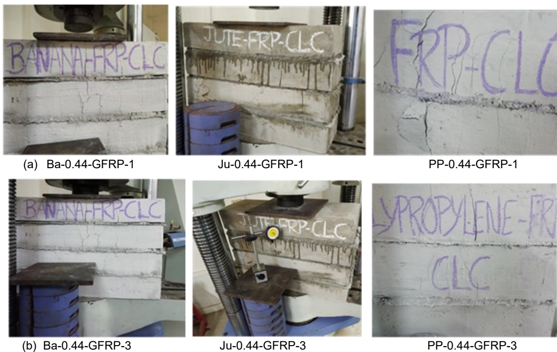
Figure 10. Failure of GFRP reinforced LWC prism with 0.44% fibers (i) 1 layer of GFRP (ii) 3 layers of GFRP
