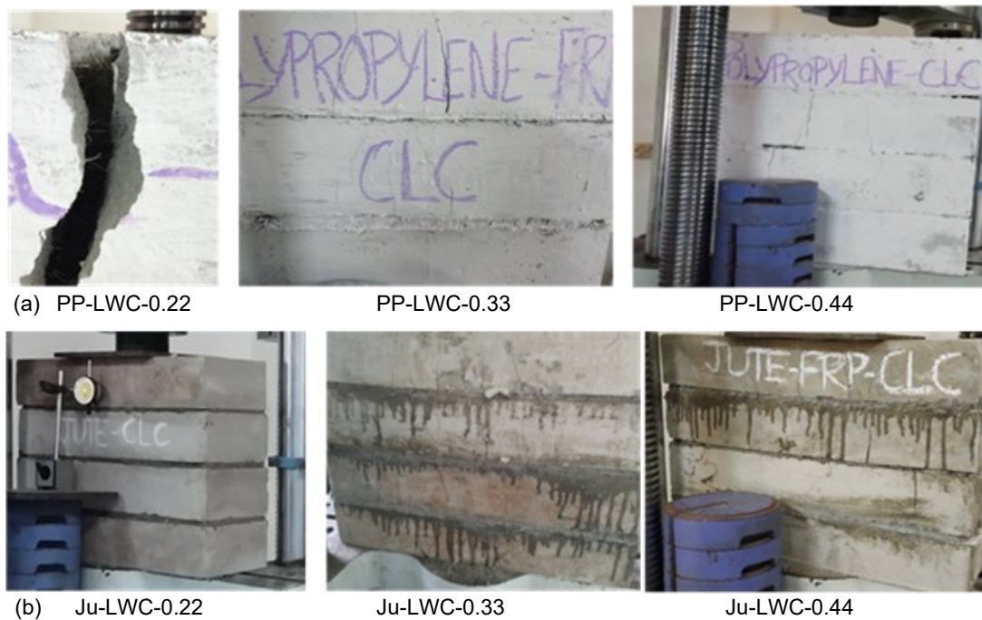
Figure 8. Failure mode of FR LWC prism (a) Polypropylene FRLWC prism (b) Jute FRLWC prism
