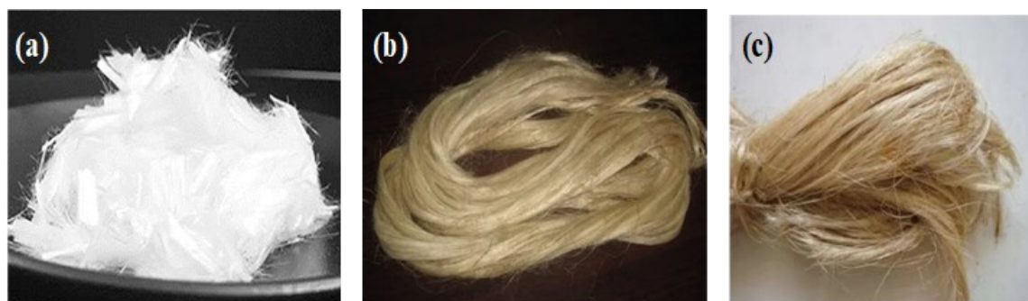
Figure 2. Fibers used in the foam concrete (a) polypropylene (b) Jute (c) Banana
