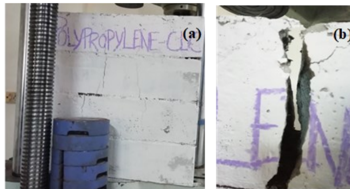
Figure 6. Crack formation in specimen (a) before peak load (b) wider crack after peak load
