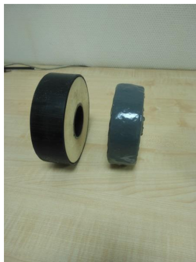
Figure 2 - Specimens of the pipe. On the left: in outer casing of polyethylene. On the right: with polyurea coating
