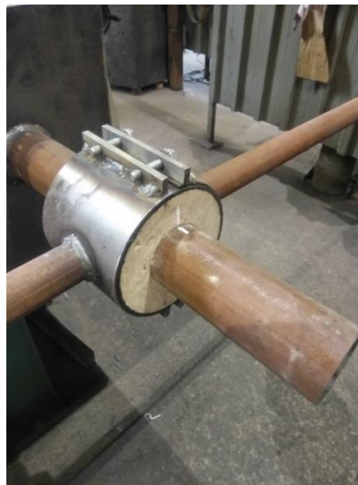
Figure 1 - Installation for determining the shear strength in the tangential direction
