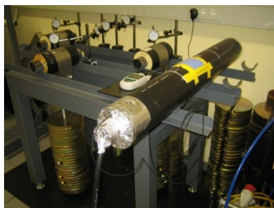
Figure 4 - Experimental setup for thermal conductivity measuring
