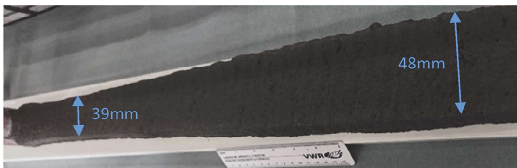
Slika 11. Konzistentnost dimenzija – variranje širine odštampalog sloja [10] Figure 11. Dimension consistency - variations in width of the printed layer [10]
