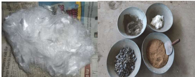
Figure 1. Polypropylene fibre and ingredients of concrete
