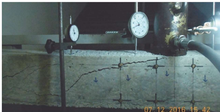
Slika 14. Mehanizam otkaza CRC modela Figure 14. Mechanism of CRC model failure
