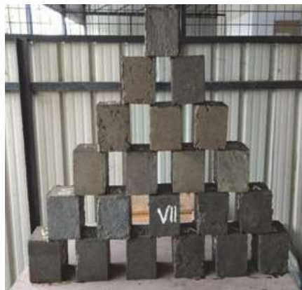
Figure 2. Test Specimens to measure compressive strength
