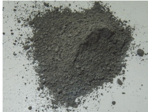
Mixed wheat straw and sunflower husk ash, after sieving and grinding
