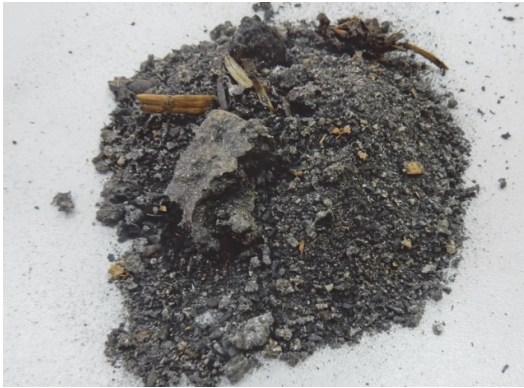
Mixed wheat straw and sunflower husk ash, before sieving and grinding
