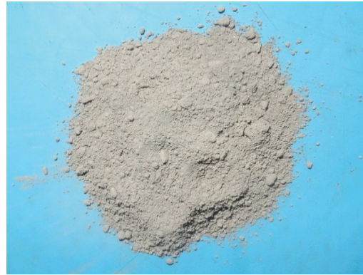
Oil rapeseed ash, after sieving and grinding
