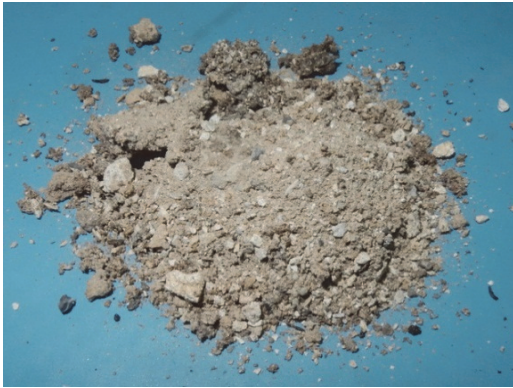
Soya straw ash, before sieving and grinding
