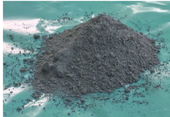
Wheat straw ash, after sieving and grinding
