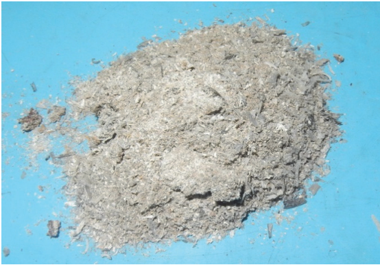
Oil rapeseed ash, before sieving and grinding
