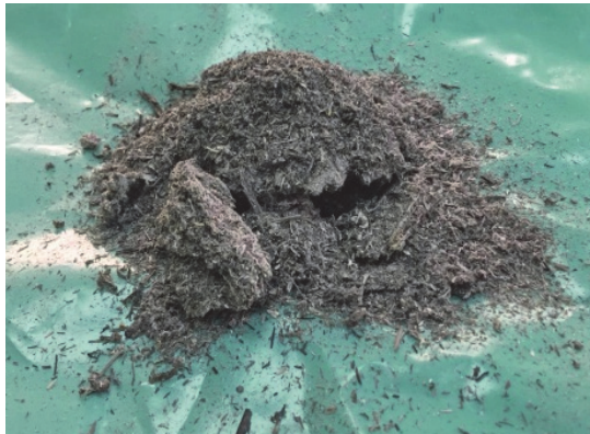
Wheat straw ash, before sieving and grinding
