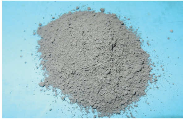
Silo waste ash, after sieving and grinding
